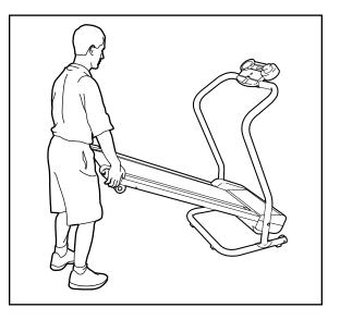
2. Move your right hand to the position shown and hold the treadmill firmly. Raise the treadmill until the latch pin is aligned with the hole in the left handrail. Slide the latch pin into the hole. Make sure that the latch pin is inserted as far as possible into the hole. Lock the pin by pressing the end of the pin into the slot in the storage latch as shown in the inset drawing.
